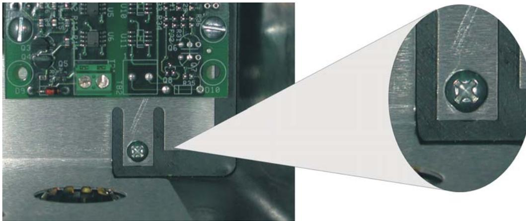
Accessible screw for securing shields to earth ground
